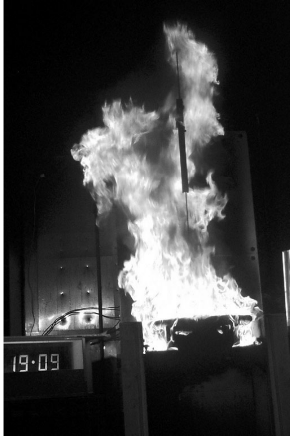
Figure 2. Accelerating flaming combustion observed during the testing of some decking materials.
