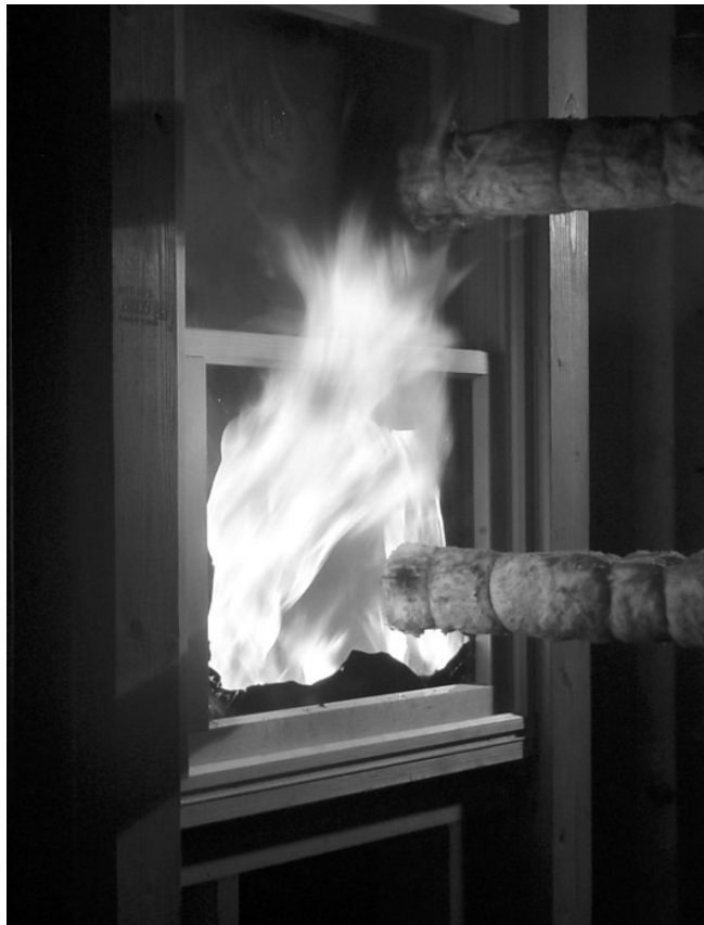
Figure 7. Glass breakage as a result of the flame exposure.
